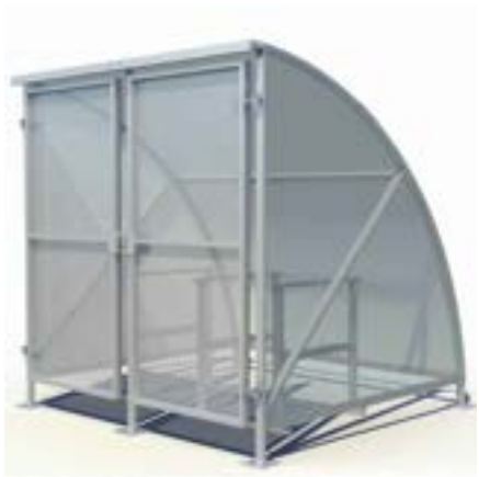
GALVANISED STEEL FRAMED CYCLE STORAGE SHELTER, FOR 6 CYCLES, 2150mm LONG x 2000mm WIDE x 2200mm HIGH, GATED FRAMES TO RECEIVE PERFORATED INFILL PANELS. PROVIDE 3no SHEFFIELD STANDS, FIXED TO TO HARD STANDING.
