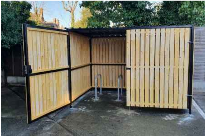
TRINITY TIMBER WOODEN BIKE SHELTER FOR SECURE SAFE STORAGE FOR 6 CYCLES. MADE FROM 50x50x3mm MILD STEEL BOX FRAME, WITH ROUGH SAWN TIMBER CLADDING, AND DOUBLE DOOR OF TIMBER CLADDING WITH 3 HINGE ANTI-LIFT DOORS. BEING 2350mm DEPP AND 2650mm WIDE, AND A HEIGHT OF 2150mm HIGH. WITH 3 NO SHEFFIELD TOAST RACK, SECURE DOWN TO CONCRETE BASE.
