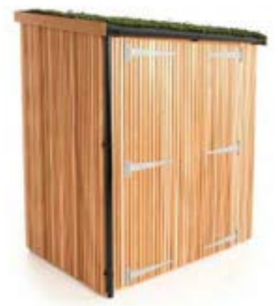
VERTICAL TIMBER BIKE SHELTER FOR SECURE SAFE STORAGE FOR 6 CYCLES. MADE FROM TIMBER FRAME, WITH ROUGH SAWN TIMBER PANELING, AND DOUBLE DOOR OF TIMBER CLADDING WITH 3 HINGE ANTI-LIFT DOORS. BEING 1300mm DEEP AND 2600mm WIDE, AND A HEIGHT OF 2200mm HIGH. WITH METAL RACKING TO SECURE BIKES TO VERTICALLY.
